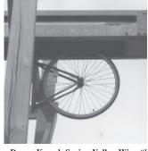
Duane Kuesel, Spring Valley, Wis.: "I have a silage conveyor belt that's more than 100 ft. long. Occasionally the belt will slip on the drive hub without my knowing it. One time the belt slipped for such a long time that it burned completely through. That's when I came up with the idea for a bicycle tire monitor. The tire is always in contact with the moving belt, which rotates the tire. As a result, I can tell at a glance if the belt is working properly. I cut down part of the bike frame
