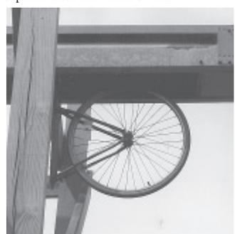
**Duane Kuesel, Spring Valley, Wis.:** "I have a silage conveyor belt that's more than 100 ft. long. Occasionally the belt will slip on the drive hub without my knowing it. One time the belt slipped for such a long time that it burned completely through. That's when I came up with the idea for a bicycle tire monitor. The tire is always in contact with the moving belt, which rotates the tire. As a result, I can tell at a glance if the belt is work-
