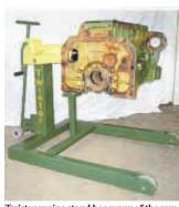
Twister engine stand has many of the same features found on larger engine stands. Rd. 550 E., Greensburg, Ind. 47240 (ph 812 663-8567; fax 812 663-8698; kssteel@aol. com).
