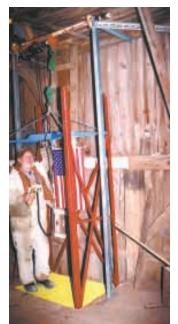
Gene Boehler needed a way to take big parts and other items up to the loft storage area in his shop, so he built this eleva-tor. It can lift up to 900 lbs. and rides up through an existing opening in the hayloft floor.
