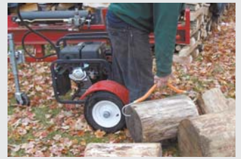
One-handed firewood gripper has two hooks with a handle in between.
