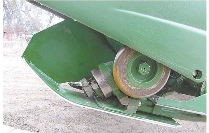
One of the skid shoes on Gutschmidt's Deere 630 Hydra Flex combine header kept pushing up mud and dirt. To solve the problem he flattened the shoe to more of a gradual incline.
