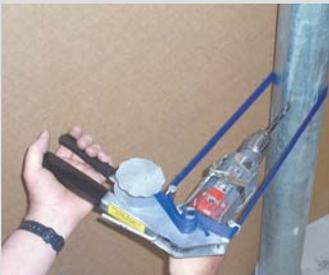
drills and allows you to put as much pressure as you want on the drill bit simply by squeezing the ratchet. Works great in many difficult-to-drill applications.
