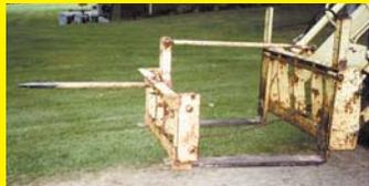
I figured out how to mount a hay spear on my front-end loader without taking off the set of forks I normally have on there. The forks simply slip into brackets at the bottom of the rectangular frame and a metal rod brace at the top runs back to the loader frame. Works great handling round bales. You just have to have a tractor with enough weight to balance out the bale. **(Albert V. Dalton, 103 Dalton Circle, Ridgeway, Va. 24148)**
