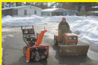
Tecumseh snowblower to use but found that his faithful old 3-speed Montgomery Wards lawn tractor does just as well with a home-built plow attachment on front. He made it by simply fastening an old metal cabinet door to the front-end hitch attachment on the tractor, bolting it to angled braces that tilt the plow slightly to push snow to the side. It works faster than the snowblower to clear large areas and he still has the snowblower for everything else. **(Jack Danahy, Greenfield, N.Y.)**
