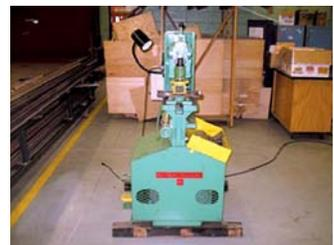
ironworker (www.unihydro.com). "I use it to cut, punch, and bend metal and to do many other jobs. It cuts my repair time in half and works great. After 20 years of use it's still worth within about \$500 of a new one."
