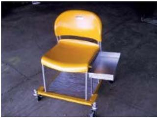
**Don Blake, Cherokee, Iowa:** "I used an old chair and some scrap steel to make a handy roll-around shop chair that holds tools and parts. It really makes it easier for an old man to work on machinery."
