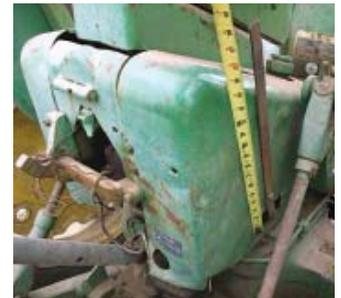
while looking back over my right shoulder. The lift lever was previously mounted on the dash and would often get stuck. I moved the lever to the back of the tractor.
