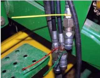
put colored plastic ties on the hydraulic hoses and valves to make it easy to hook up the right hoses. It's a cheap replacement for the colored plastic covers that come on the hoses but often get ripped off and lost. You can buy a whole box of ties for a couple dollars."
