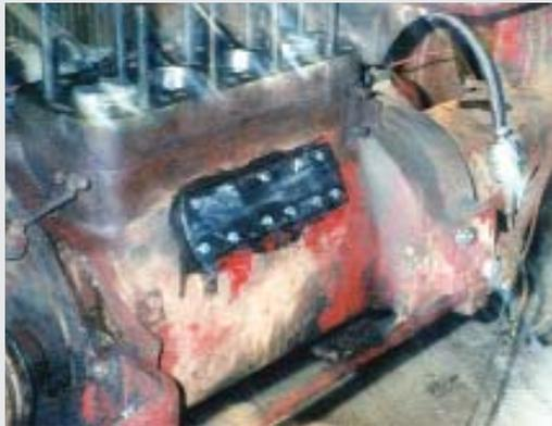
Engine Block Repair Patch
