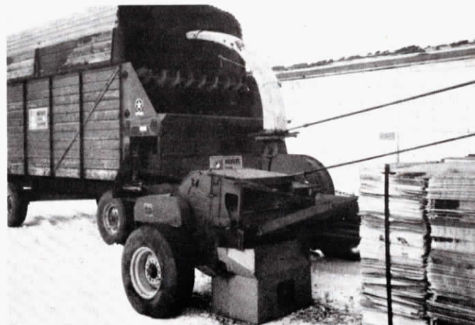
Kraemer uses a Deere chopper to turn old newspapers into bedding for livestock.
