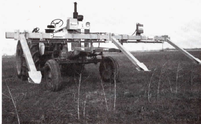
Weeds break the electric beam between the extended arms, triggering the sprayer which sprays the weeds, then shuts off automatically.
