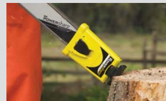
Sharpener snaps onto end of chainsaw bar. To activate, start saw and press "foot" against a hard surface (below).
