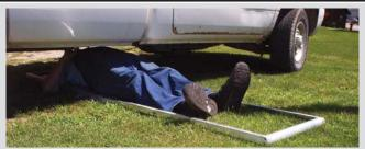
Creeper has a 4-ft. long movable bed that rolls on wheels inside an 8-ft. long metal frame. You just slide yourself under the vehicle.
