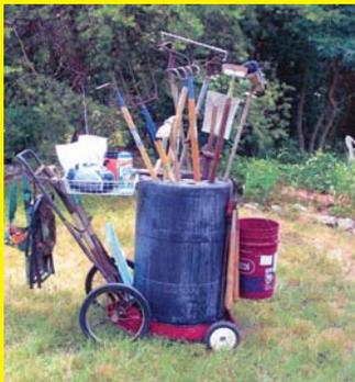
drilling holes in the top to hold shovels, rakes and other long-handled tools. A hook on front holds a 5-gal. pail and a wire shelf attaches to hangars between the drum and the push handle. Tools, cords and other items hang off the push handle. It's a simple idea that saves a lot of time running back and forth. You could never carry all these tools in a wheelbarrow. **(Lewis P. Tomlin, 16391 Gun Barrel Road, Montpelier, Va. 23192)**
