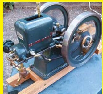
I enjoyed building this 1/4-scale model of a 1912 Red Wing 5 hp "hit and miss" engine. It runs well with ignition provided by a Ford buzz coil and a spark plug.
