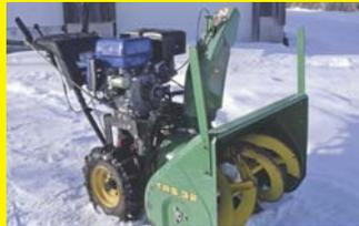
The drive unit on my Deere walk-behind snowblower kept breaking down. I replaced the drive with a hydrostatic unit from an Uber feed cart. A Cub Cadet transmission would also work. The frame of the snowblower was too small so I used 2-in. angle iron to build a platform to support the new drive unit. It worked great - lots of power. **(Phillip Krywosa, Boonville, N.Y.)**
