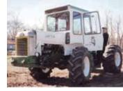
metal to build the frame. It has air brakes and power steering and a 5-speed transmission with a 4-way 2-speed Brownie, which gives me 40 forward gears. I already had the wheels and got the cab from a salvage yard."
