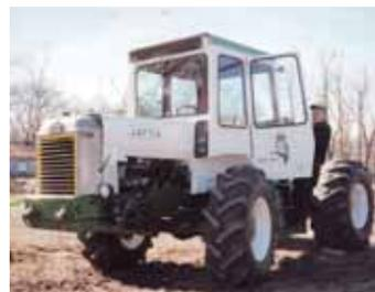
metal to build the frame. It has air brakes and power steering and a 5-speed transmission with a 4-way 2-speed Brownie, which gives me 40 forward gears. I already had the wheels and got the cab from a salvage yard."
