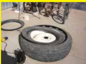
We needed turf tires for our tractor but could not justify them. So we bought some old, bald truck tires that were 1/2 size bigger than the tractor tires. We cut 2 to 2 1/2 in. off the inside of each tire sidewall and slid them onto the tractor tires, then reinfated. Works great and we no longer leave tracks from lugged tires when spraying weeds. (Andy, Delta, Colo.)
