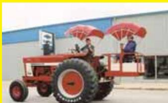
tractor for parades, tractorcades, or crop tours. It attaches to the tractor's 3-pt. hitch and has a sun shade, easy step, and an entry door with an air-ride seat. It's made from heavy-duty steel with white plywood trim to match the tractor. (Dennis Neubauer, 31491 Co. Hwy. S27, Garden City, Iowa 50102, ph 515 893-2320)
