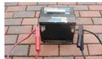
When his portable jump start battery went bad, Larry Wood bolted the battery cables to a side post car battery.
