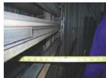
Storage rack is fitted with 43 individual boxes welded about 8 in. apart on 4 lengths of 100-ga. chain.
