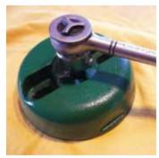
Tool fits on a 1/2-in. drive socket and allows you to rotate the crankshaft on Deere 2-cyl. tractors, without having to remove the flywheel cover.
