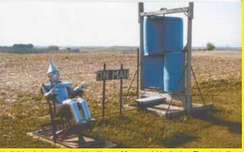
I built this wind-powered rocking "tin man" for a roadside display. The windmill, on the right, is made from plastic barrels cut in half and mounted on a vertical shaft. It drives a horizontal drive shaft that runs over to the tin man's rocking chair. He looks quite content sitting there. (Louie Waelti, N3337 Aebly Road, Monroe, Wis. 53566)
