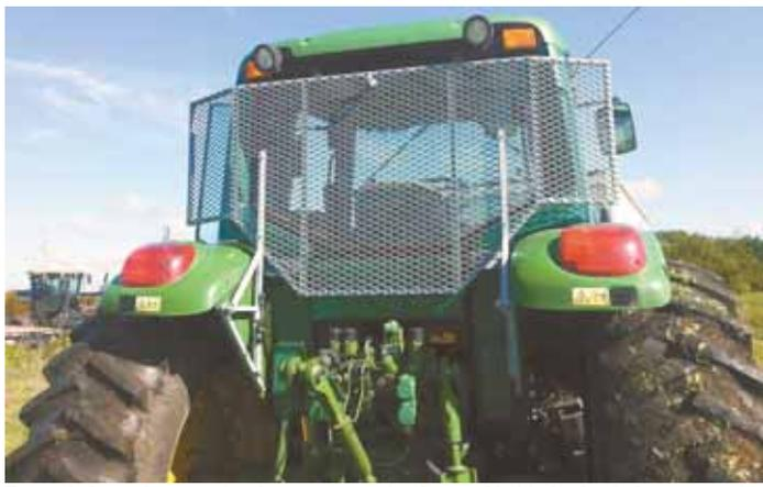
Expanded metal screen sits above tractor's fenders and behind cab window, protecting both the window and tractor operator.
