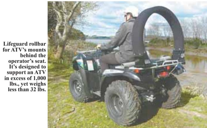
Lifeguard rollbar for ATV's mounts behind the operator's seat. It's designed to support an ATV in excess of 1,000 lbs., yet weighs less than 32 lbs.
