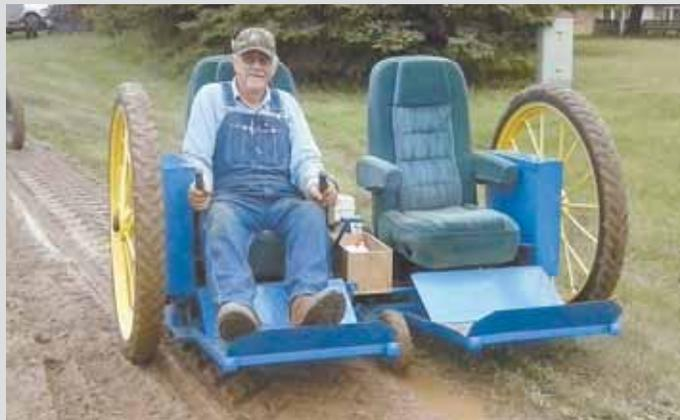
A pair of levers are used to steer. “I pull way back on both levers to stop. By pulling back on just one lever it’ll spin around in its own tracks,” says Grovom.
