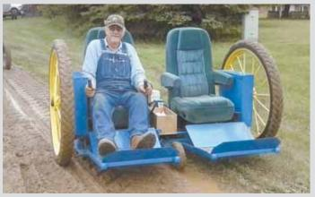
A pair of levers are used to steer. "I pull way back on both levers to stop. By pulling back on just one lever it'll spin around in its own tracks," says Grovom.
