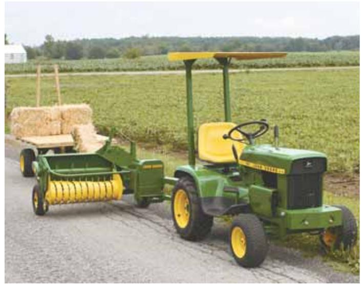
After R.W. Prinkey built a half-scale wagon, he decided he needed a baler to match. An electric motor powers the flywheel-driven pickup and plunger.
