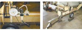
With the exception of the knotters, all major parts and drives work as they would on a real baler, and are powered by a 12-volt electric gearmotor.
