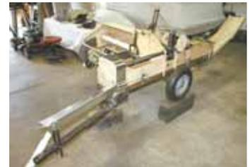
With the exception of the knotters, all major parts and drives work as they would on a real baler, and are powered by a 12-volt electric gearmotor.
