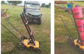
"Feed bucket carrier" is bolted to mower deck and looks like a short ladder tilted backward. It holds up to three 5-gal. buckets.
