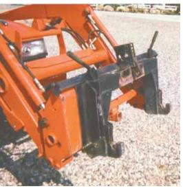
Alfred Jefferv converted a Harbor Freight 3-pt. hitch to hook up to the bucket mount on his tractor's front-end loader.
