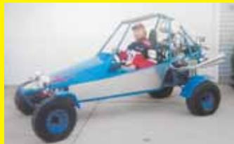
I built this Badland Buggy using a bundle of pipes, machining my own spindles and hubs. The machine is powered by a 1980 Honda CB 740 engine, and I made a reverse gearbox so I can back it up.
