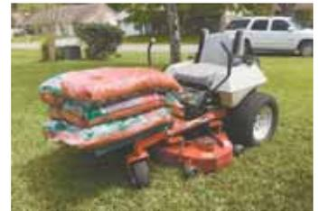
Platform is built strong enough to carry several 50-lb. bags of mulch. Putteet also installed ball hitches at both ends of machine.
