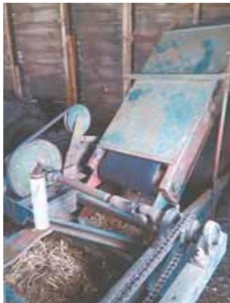
Bale thrower is chain and belt-driven off a pair of rubber-tired wheels that ride on the flywheel.
