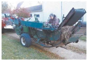
When Kevin Bahe bought this Deere/New Holland hybrid baler, a New Holland kicker had been grafted to the Deere baler with a drive unit fabricated to run off the flywheel.
