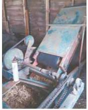
Bale thrower is chain and belt-driven off a pair of rubber-tired wheels that ride on the flywheel.
