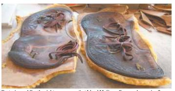
Restoring saddles the right way means that Lloyd McConnell uses only genuine fleeces. Attaching one requires laying the skirt out on a whole fleece. He marks the shape, glues the skirt in place, and trims the fleece.
