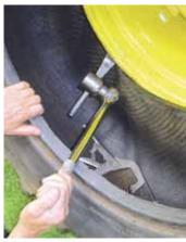
Terry Regimbal's tractor tire mounting tool makes use of a 3/4-drive ratchet and a 6-in. stub bar. Ratchet is used to pull bead down into wheel rim's drop center.
