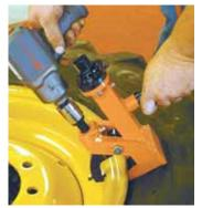
Pneu-Tek Tire Tools' Ag Kit lets you fix tires fast. All you need is an air impact wrench. Photo above shows bead breaker; below is a demounter.
