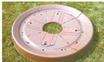
Pie-shaped sections with holes in them snap together to form a solid ring that slopes toward the center. Four adjustable "doors" snap into place on top of ring and can be used to slide the sections in or out, allowing ring to expand as tree grows from 1 to 12 in. dia.
