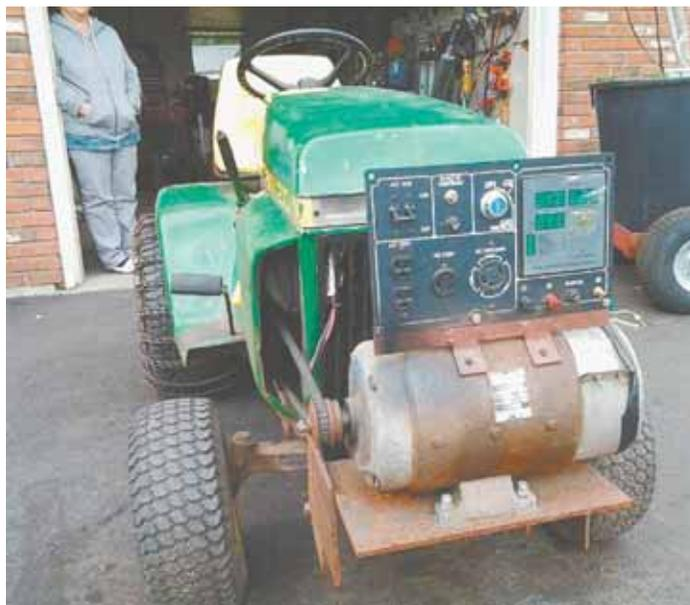
Carmin Mazzucco mounted a 7,500-watt 240/120 30-amp generator on the snowplow mounts in front of his Deere garden tractor.
