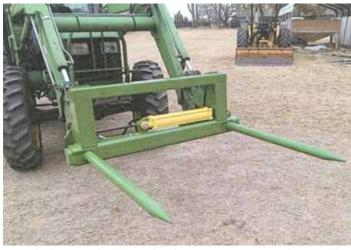
Forks slide in or out using a hydraulic cylinder attached to a telescoping tube. Width between forks is set by inserting a pin into a hole.
