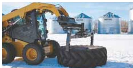
Tire Jogger uses hydraulic cylinders to grab, hold, and rotate large tires from the safety of a skid loader. Two large metal "arms" securely grip and hold the tire.
