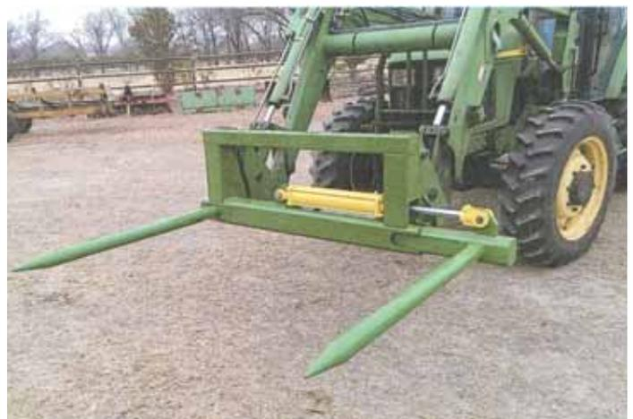
"The forks can handle round bales from 4 to 5 ft. wide. The operator can insert the forks into the bale, or grasp it from both sides to keep from damaging net-wrapped bales," says Gary Machado.
