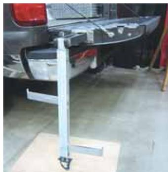
"Hideaway" tailgate steps fold out from the sides of an aluminum post, which pulls out of a tailgate tube when needed.
