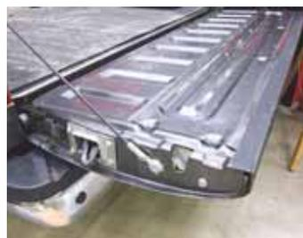
Operator grabs a nylon strap to pull step post out.
