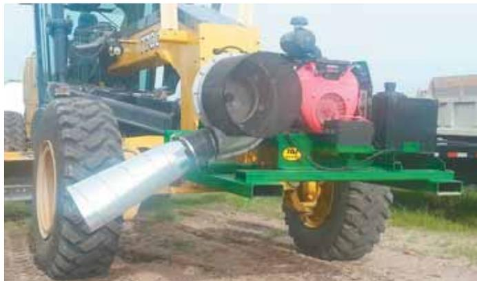
Terry Jacob blows grass clippings off road edges before blading them with the township grader. Blower is positioned ahead of grader's front wheels.
