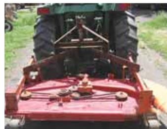
David Simpler wanted a 3-pt. mounted mower deck for his Satoh tractor so he converted a Kubota belly-mounted deck, turning the deck's gearbox 180 degrees and adapting the 3-pt. lifting mechanism from a one-row cultivator.
