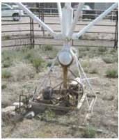
At center of walker, Rising mounted a car rear end with an axle stub mounted to a metal frame on a concrete pad.
