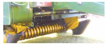
Dean Nelson got tired of seeing hay laying on the field after falling off both ends of his round baler pickup, so he attached truck mud flaps to the pickup's outside edges.
