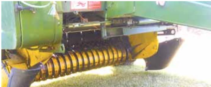
Dean Nelson got tired of seeing hay laying on the field after falling off both ends of his round baler pickup, so he attached truck mud flaps to the pickup's outside edges.
