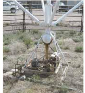
At center of walker, Rising mounted a car rear end with an axle stub mounted to a metal frame on a concrete pad.
