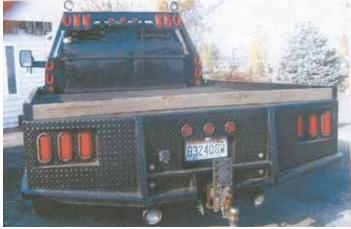
Alan Heilman fitted his Dodge 3500 1-ton dually pickup with a flatbed, that rests on two 1-in. thick steel bars.
