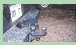
Rotating tri-ball hitch comes with 3 hitch balls in 7/8, 2, and 2 5/16-in. sizes that are welded to a steel plate.
