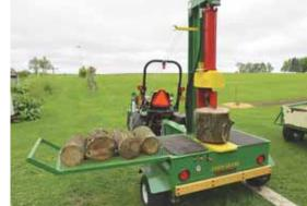
A 12-volt winch is used to raise and lower the 5-ft. long loading arm on Ed Hollmer's vertical splitter. "Very little lifting or bending is required," he says.
