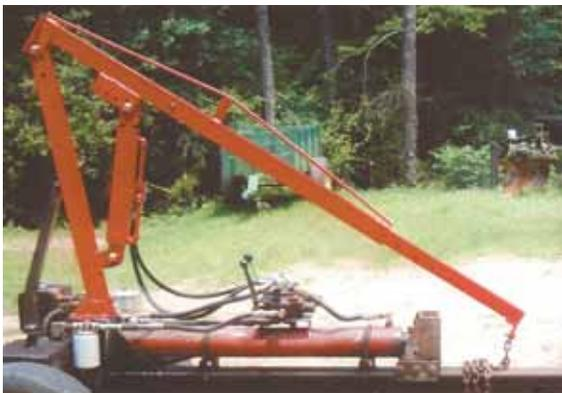
**Oliver Campbell added this boom to his log splitter, making it easy to lift big chunks into place.**
