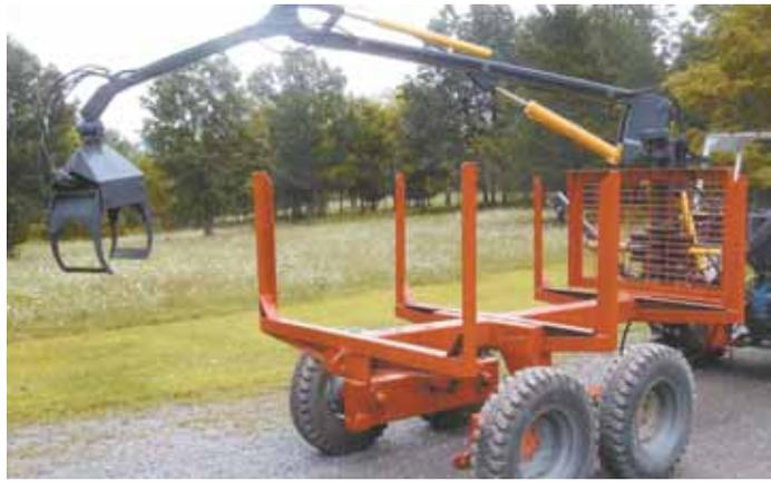
**Logs are loaded onto trailer by a grapple, which is supported by a boom that rotates on front of trailer. Boom can reach out 13 ft. and swing about 185 degrees.**
