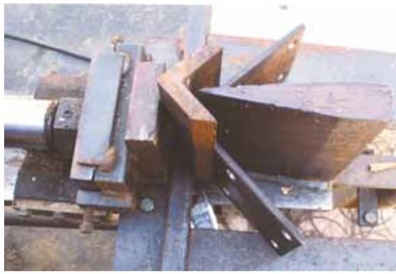
**Forrest Robinson made this press brake to fit his log splitter. “I can use 3 different V-shaped brackets with it, depending on the thickness of the metal I want to bend,” he says.**
