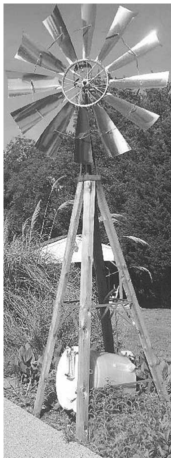
Mark MacLean turned a junked bicycle and the drum from an old washing machine into this wind-powered compost tumbler.
