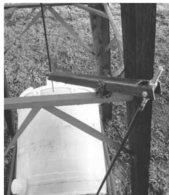
As pole pushes down, it cranks a horizontal shaft that slowly rotates drum.
