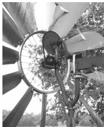
Windmill's blades are bolted to rear wheel rim off a bicycle. Bike's pedal is connected to a vertical shaft that fastens to drum.
