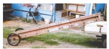
Tom Kalista attached a pair of lawn mower wheels to the bottom of his extension ladder, making it easier to move around.
