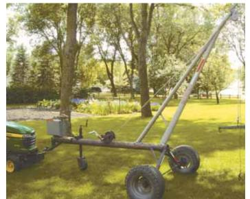
Mini crane rides on a pair of old car tires and attaches to ball hitch on Miner's garden tractor. Lifting is done by a pair of manually-operated, side-by-side winches.
