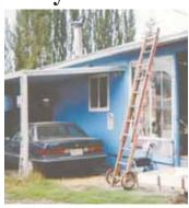
When the ladder is up against a building, the wheels are off the ground.
