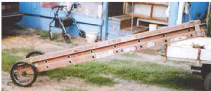
Tom Kalista attached a pair of lawn mower wheels to the bottom of his extension ladder, making it easier to move around.
