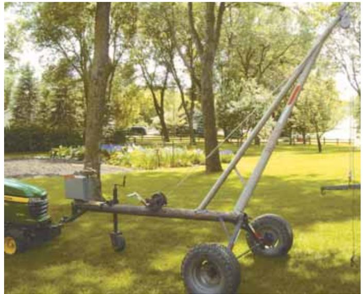
Mini crane rides on a pair of old car tires and attaches to ball hitch on Miner's garden tractor. Lifting is done by a pair of manually-operated, side-by-side winches.
