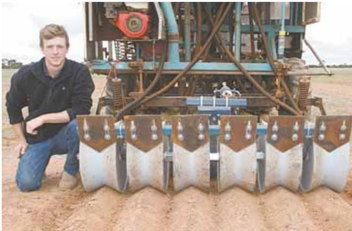
Wesley Wheel uses specially-designed tillage points and V-shaped metal wheels to make raised beds. The shallow furrows collect water as it runs off beds.
