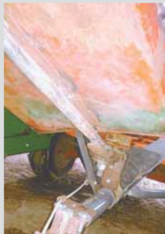
Steve Schultz modified his baler's chute so it would follow with his E-Z Trail Bale Basket more closely. He keeps the pan turning with the Bale Basket with the aid of a 3/4-in. steel rod that rides inside a pipe.
