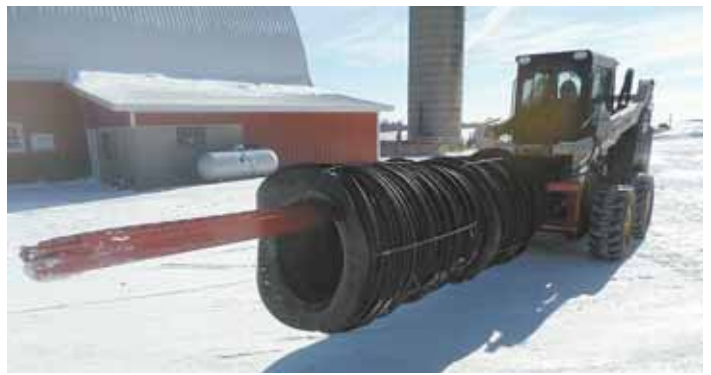
A track and chain is used to move tires on and off unit's 16-ft. steel boom. Boom raises up to a 20-degree angle.
