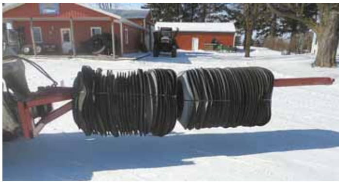
Skid loader-mounted "shooter" works great for putting tires on silage piles and bunkers, and for loading and unloading tires on trucks and trailers.
