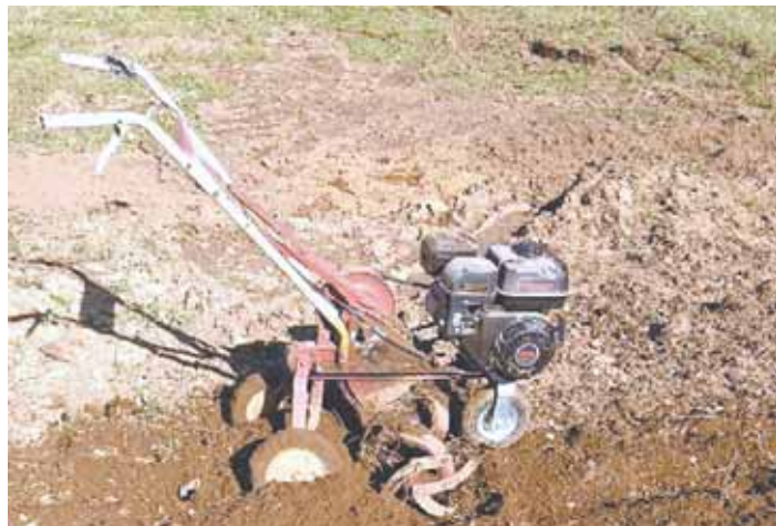
Jared Wagoner added a 10-in. dia. pneumatic caster "gauge wheel" to his Snapper front tine tiller, to keep it from digging too deep in loose soil.
