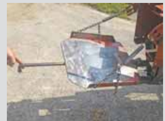
Steve Schultz modified his baler's chute so it would follow with his E-Z Trail Bale Basket more closely. He keeps the pan turning with the Bale Basket with the aid of a 3/4-in. steel rod that rides inside a pipe.
