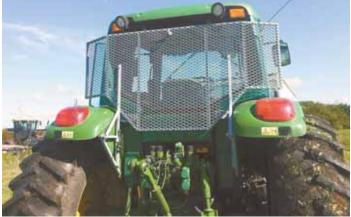
Expanded metal screen sits above tractor's fenders and behind cab window, protecting both the window and tractor operator.
