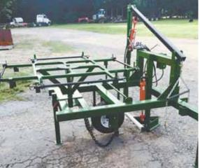
Dennis Trussell's 3-pt. mounted poly pipe layer digs the trench, lays the pipe, and partially covers it in one pass.
