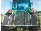
Fender-mounted brackets allow screen to pivot down for cleaning or opening the window.
