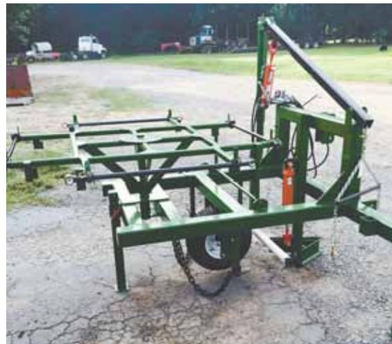
Dennis Trussell's 3-pt. mounted poly pipe layer digs the trench, lays the pipe, and partially covers it in one pass.
