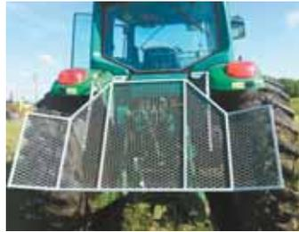
Fender-mounted brackets allow screen to pivot down for cleaning or opening the window.
