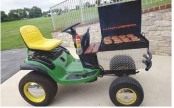
Dale Clugston's barbeque grill mounts in place of the engine on his Deere lawn tractor. Power to move the mower is supplied by a 12-volt electric motor.
