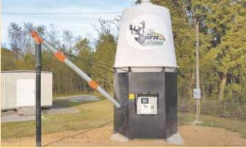
Corn Xpress is a giant vending machine that dispenses fresh corn on demand. An unloading auger feeds into trucks, trailers, or buckets.
