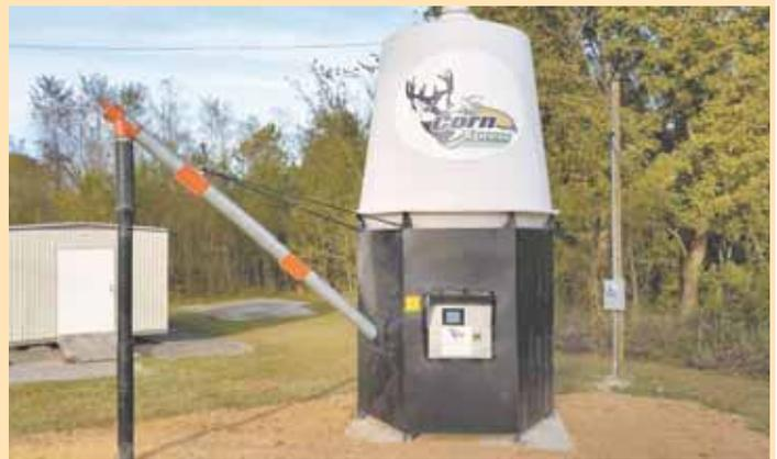
Corn Xpress is a giant vending machine that dispenses fresh corn on demand. An unloading auger feeds into trucks, trailers, or buckets.
