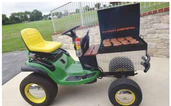
Dale Clugston's barbecue grill mounts in place of the engine on his Deere lawn tractor. Power to move the mower is supplied by a 12-volt electric motor.
