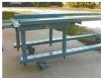
Vern Goodwin needed a hoist to help mount a sidecar on a motorcycle, so he built this table hoist. "It lets me put the sidecar in the exact place and height I need," he says.
