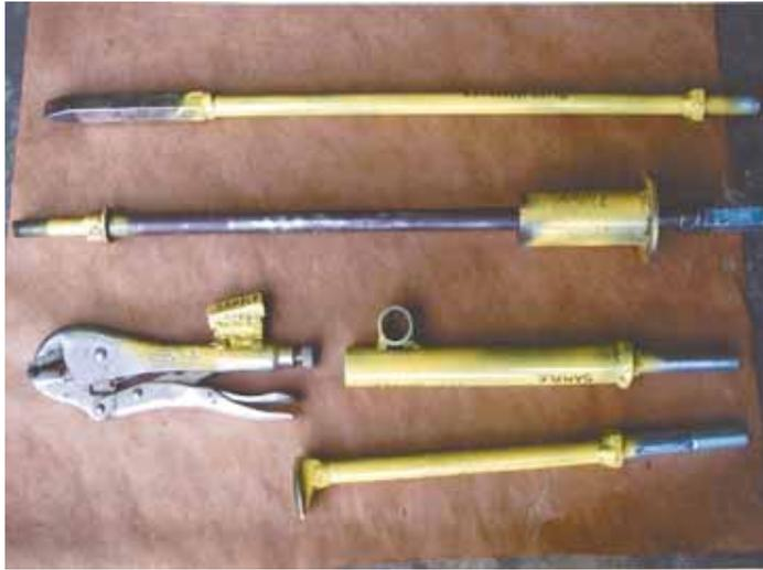
Slide hammer (second from the top) attaches to several tools including a chisel, vice-grips, post puller and hammer.
