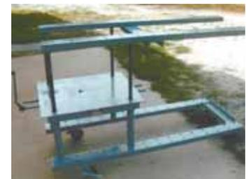
"The sidecar fits onto the top frame," says Goodwin. "We put it on there, roll it into position next to a bike, then raise it and level it next to the bike."
