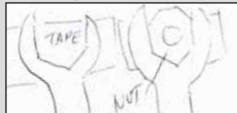
**Oran G. Underdahl, Fosston, Minn.:** "When I have to get a nut on a bolt in a tight spot that I can't reach with my fingers, I put sticky tape across the opening on the wrench. Then stick the nut to it. You'll be able to get it started."
