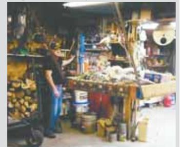
**Dean Wallace, Oconee, Ill.:** He set up a temporary hanging storage box that he can raise or lower as needed. It measures 4 by 6 ft. and hangs from the ceiling on four flat steel bars. The bars pivot freely on bolts at each corner. An electric winch cable pulls the shelf up from one end, pivoting to the side to lift up. Dean just flips a switch on the wall to raise or lower the shelf.
